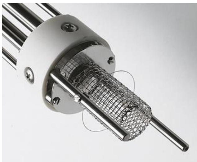
Figure 1. SRS electron impact ion source for RGA applications used for the simulation model. The wired structure is the anode cage and the thin round wire around it is the thermionic electron emission filament (cathode). The ion outlet is directed to the upper left corner. Picture taken from www.thinksrs.com .
