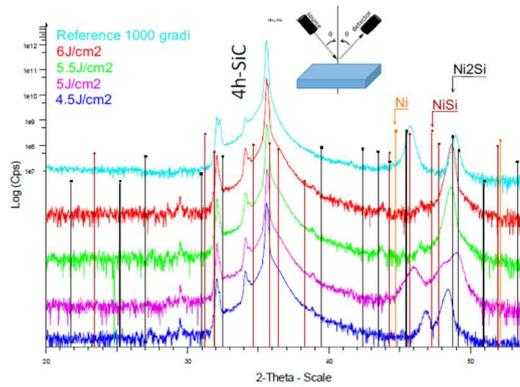
**Fig. 2.** XRD patterns in symmetric configuration of Ni samples annealed at different fluence with double scan process, compared with standard RTA pattern. Ni<sub>2</sub>Si peaks are observed for all three laser annealed samples.
