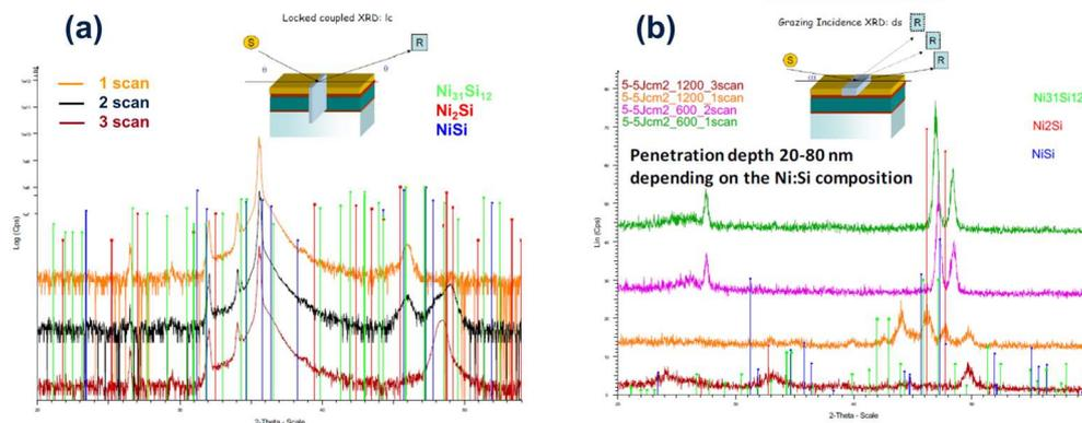
**Fig. 1.** (a) XRD patterns in symmetric configuration of the Ni samples annealed at  $5.5 \text{ J/cm}^2$  of fluence for single, double and triple scan process. With increasing of scan number, a shift towards Si rich phases is observed. (b) XRD patterns in grazing incidence configuration of the Ni samples annealed at  $5.5 \text{ J/cm}^2$  of fluence for single and triple scan process.  $\text{Ni}_{31}\text{Si}_{12}$  peaks are observed in both samples.
