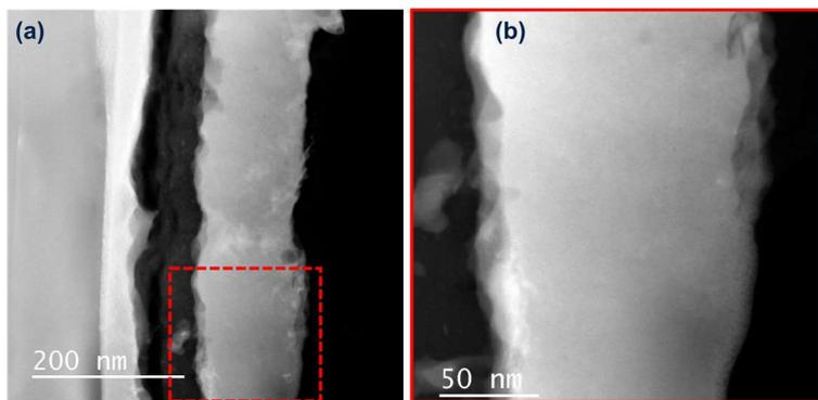
**Fig. 3.** Cross sectional TEM images of the Ni sample annealed with double scan at 6 J/cm<sup>2</sup>, showing a continuous layer of C-clusters close to the interface between SiC substrate and reacted layer (a) and the absence of C-clusters outside of this region (b).
