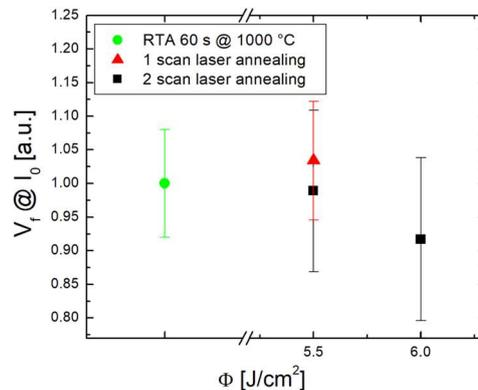
**Fig. 4.** Forward voltage ( $V_f$ ) of diode at nominal current as a function of fluence and scan number of laser annealing process, compared with standard RTA results. Increasing of fluence and multiple scan play a crucial role in  $V_f$  reduction.
