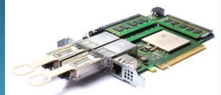
High data rate data grab module developed by PRODRIVE
